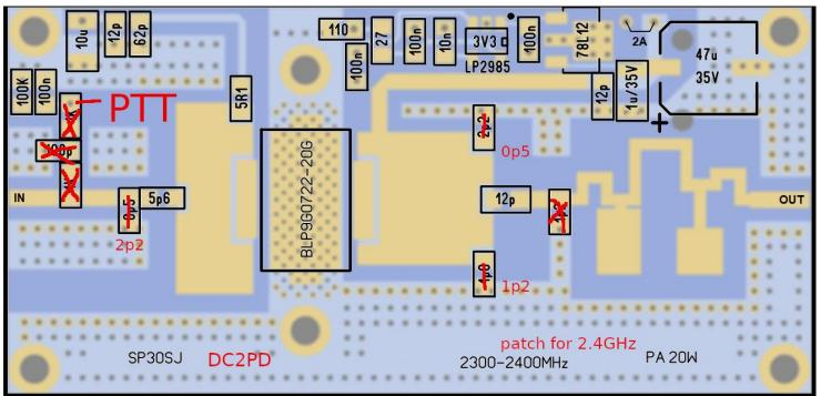
I have build your PA with your PCB, but I run into some problems. The provided output match has a maximum at 2.1GHz and falls down -13 dB to 2.4GHz. The design looks like the test circuit for 2.1Ghz from the datasheet. I was able to get a much better match for 2.4GHz by changing the existing ATC caps.
